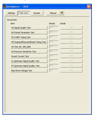
2. Click the [LS Upstream Signal Quality Test] button in the dialog box. The Device LS Upstream Signal Quality Test dialog box is displayed.
