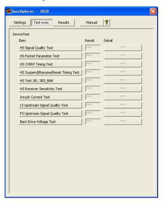
**2.** Click the **[HS Signal Quality Test]** button in the dialog box. The Device HS Signal Quality Test dialog box is displayed.
