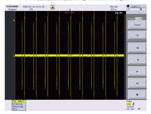
**19.** Confirm that a 12-bit Sync field is received from the data generator, and confirm that NAK is returned from the DUT (EL\_18).
