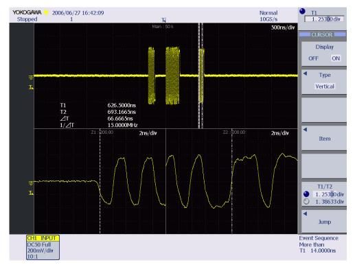
16. Confirm the Sync field of the 3rd packet (from device)(EL\_21). Using the digital oscilloscope's zoom function, adjust the zoom position on the 3rd packet. Then set the cursors of the digital oscilloscope on the start and the end points of the Sync field of the 3rd packet (from device). The Sync field must be 32bits. When [Next] button is clicked, the measured value is judged and Fail message will be displayed if the result is failed.
