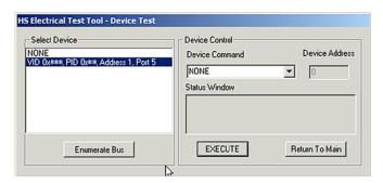
14. Click the [Next] button in the dialog box of the busXplorer-USB. Select SUSPEND from the Device Command drop down menu in the HS Electrical Test Tool, then click [EXECUTE] button.
