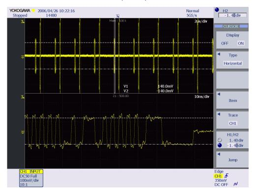
24. Click the [Next] button in the dialog box of the busXplorer-USB. To measure the squelch sensitivity level (EL16), adjust the DG2040 Data Generator's output level while watching the digital oscilloscope screen. Reducing the level of the amplitude of the packets from the data generator in 50 mV steps, adjust the output amplitude of CH0 and CH1 of the data generator to keep them the same levels until the receiver just stops responding with NAK. This is the receiver's squelch level.
