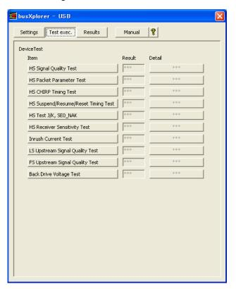
**2.** Click the **[HS Receiver Sensitivity Test]** button in the dialog box. The Device HS Receiver Sensitivity Test screen is displayed.
