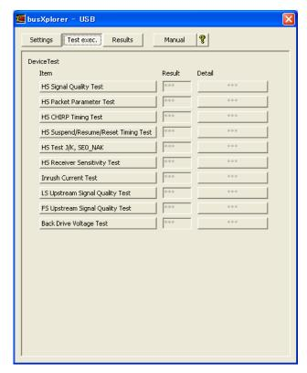
2. Click the [Inrush Current Test] button in the dialog box. The Device Inrush Current Test dialog box is displayed.
