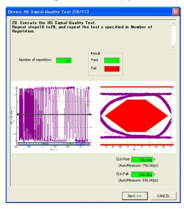
24. Click the [Next] button of the dialog box of the busXplorer-USB, repeat steps 19-23, and execute the test the number of times specified in "Number of Repetition." repeat steps 19 to 23, and repeat the test's specified in Number of Repetition.
