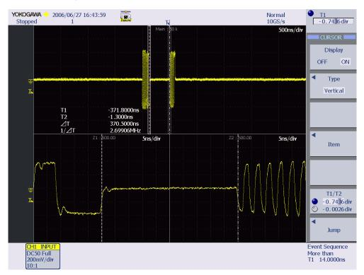
**21.** To measure the gap between packets (EL\_22), adjust zoom1 position to the end of the first packet (from host) and zoom2 position to the start of the second packet (from device).
