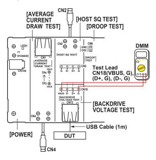
12. Click the [Next] button in the dialog box of the busXplorer-USB. Using a digital multimeter, measure the Vbus, D+ and D- voltage after Enumeration. Then input them to the text boxes in the dialog box. All voltages must be less than or equal to 400 mV.
