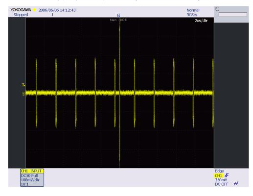
25. Click the [Next] button in the dialog box of the busXplorer-USB, and then set cursors on the Zero to Positive voltage and Negative voltage of the packet. Using zoom function of oscilloscope, adjust zoom magnitude and position so that the packet is displayed in it. Set H1 cursor on the positive peak and H2 cursor on the negative peak of the packet.
