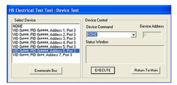
15. Click the [Next button] in the dialog box of the busXplorer-USB, select VID of DUT from the Select Divice list, then select LOOP DEVICE DESCRIPTOR from the Device Command drop down menu in the HS Electrical Test Tool, then click the [EXECUTE] button.
