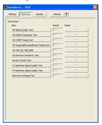
2. Click the [HS CHIRP Timing Test] button in the dialog box. The Device HS CHIRP Timing Test dialog box is displayed.
