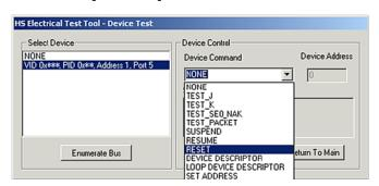
**27.** Click the **[Next]** button in the dialog box of the busXplorer-USB, check the digital oscilloscope screen to confirm that a trigger activates and the CHIRP signal is displayed.
