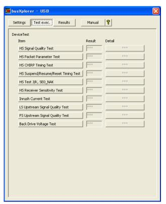
**2.** Click the **[HS Packet Parameter Test]** button in the dialog box. The Device HS Packet Parameter Test dialog box opens.
