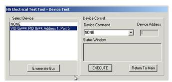
16. Click the [Next] button in the dialog box of the busXplorer-USB, and then select TEST\_SE0\_NAK from Device Command drop down menu in the HS Electrical Test Tool, then click the [EXECUTE] button.
