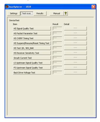
2. Click the [FS Upstream Signal Quality Test] button in the dialog box. The Device FS Upstream Signal Quality Test dialog box is displayed.
