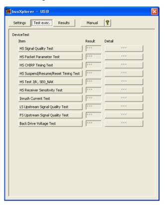
2. Click the [HS Suspend/Resume/Reset Timing Test] button in the dialog box. The Device HS Suspend/Resume/Reset Timing Test dialog box is displayed.
