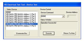
15. Click the [Next] button in the dialog box of the busXplorer-USB, select VID of DUT from the Select Device list, then select LOOP DEVICE DESCRIPTOR from the Device Command drop down menu in the HS Electrical Test Tool, then click the [EXECUTE] button.
